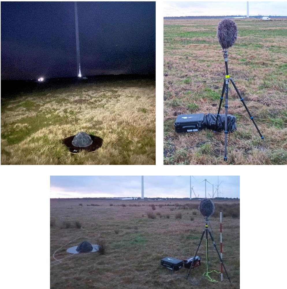
Figure 2: Microphone positions and setup. On the top left is the IEC reference position, on the top right is the tripod at 800 m and on the bottom, the two microphones at 500 m.
