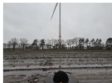
Figure 3: Picture of the microphone board used for the IEC 61400-11 test of the Enercon E160 turbine.
