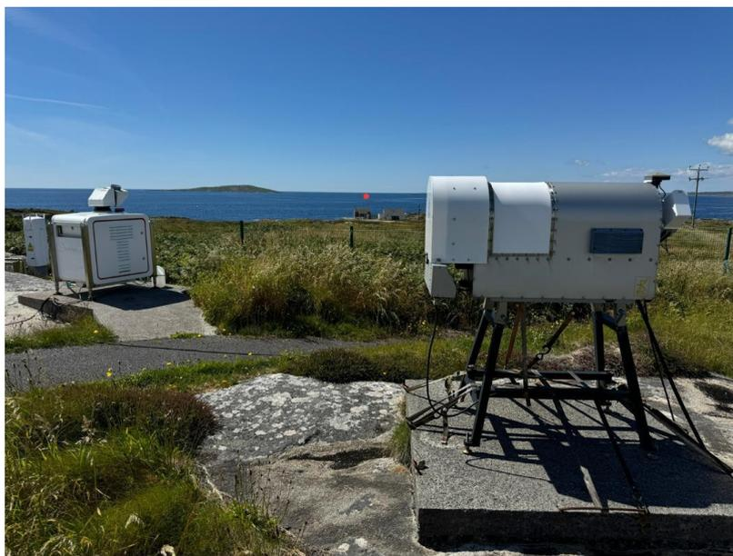
*Figure 2 Wind Profiler (Left,) IR Radiometer (Right) and Offshore Buoy (Central Red Dot)*
