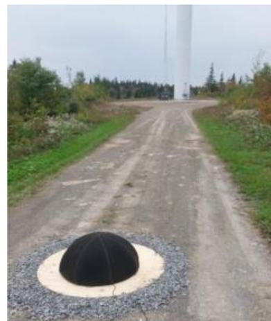
Figure 2: Picture of the microphone board used for the IEC 61400-11 test of the Senvion MM92 turbine.
